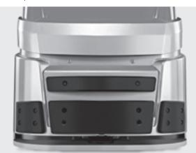
Maximum safety in series: the pedestrian protection system (PPE) actuates the emergency stop in potentially dangerous situations
