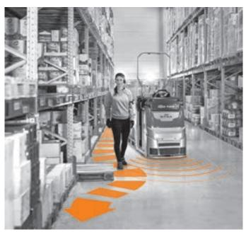
Precise handling in the event of obstacles: the OPX iGo neo autonomously avoids obstacles and reacts to the situation. Trucks will either drive around the obstacle, avoid it by driving in convoy, or – if the obstacle completely blocks its path – the truck will stop.
