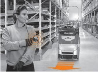
Process reliability – even for empty racks or crossroads: the OPX iGo neo recognises and passes by empty racks. Crossroads are also detected well in advance and the truck will only drive autonomously over them once the driver has checked the way is clear and has approved the onward journey.
