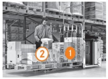
High-performance order picking: the operator can specify whether the truck moves to the first or second pallet position or anywhere in-between.
