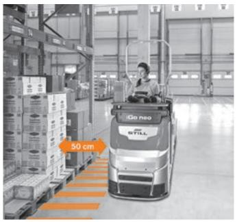
Execution of individual order picking preferences: simply stop OPX iGo neo in the desired position. The truck will stop autonomously at the exact distance from the rack as specified by the operator. If a safe distance of 500 mm is not maintained, the truck will rectify this once it is restarted. The relative position of the truck to the operator and the rack orientation can be adjusted remotely, thereby reducing walking distances.
