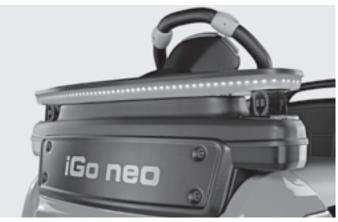
Always well informed: LED signal units indicate the current operating mode of the vehicle to the operator
