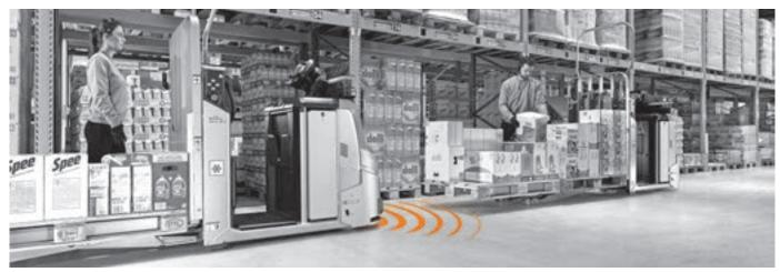
Speed is adjusted to the surroundings: if a slower truck is moving in front, or if a queue forms, the OPX iGo neo will intelligently adjust its speed to the situation. If the operator decides to travel on foot while the truck waits in the queue, then the truck will autonomously start driving again once the queue has resolved itself.
